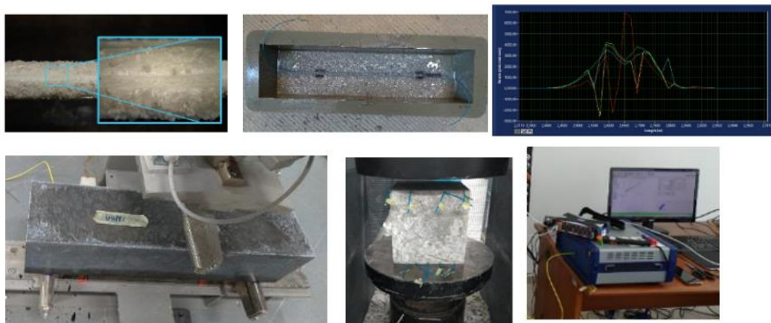
Figure 10 Acquired signal from SHM system inside UHPC concrete beam in different instants of loads.
