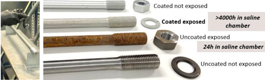
Figure 7 Direct application by spray gun of the anticorrosion coating as well as relevant results obtained after long-range exposure to saline mist chamber on real fastening elements from TSF.
