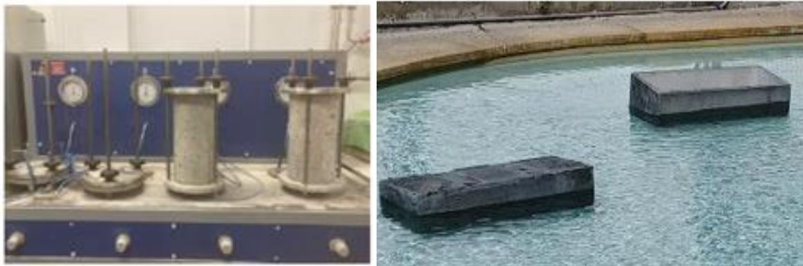
Figure 9 Small prototypes performed in preliminary trials to check production process and buoyancy.
