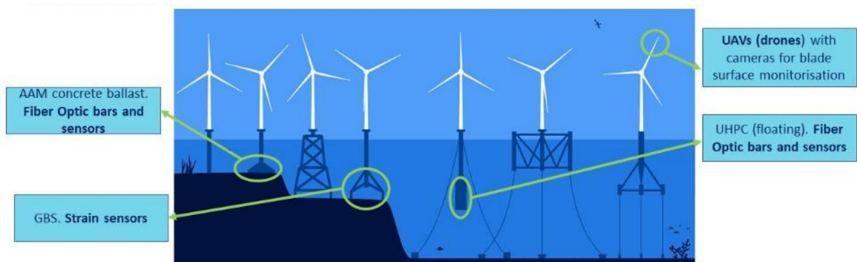
Figure 4 Main action points related to Structural Health Monitoring within MAREWIND project.
