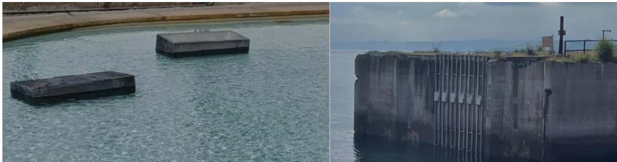
Figure 5: Floating design of UHPC structure validation for the manufacturing of the relevant scale prototype for its testing in the wave basin at EUMER facilities and real environment durability testing of UHPC at ACCIONA Harbour demosite.
