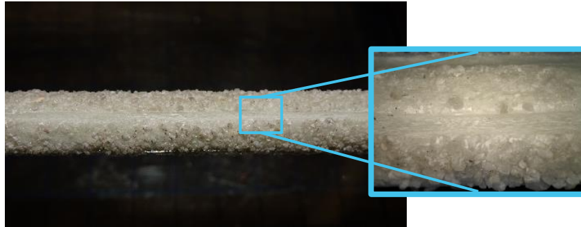
Figure 2: Groove on an improved superficial adherence GFRP rebar; in the light - blue inset an optical microscope image of the groove.
