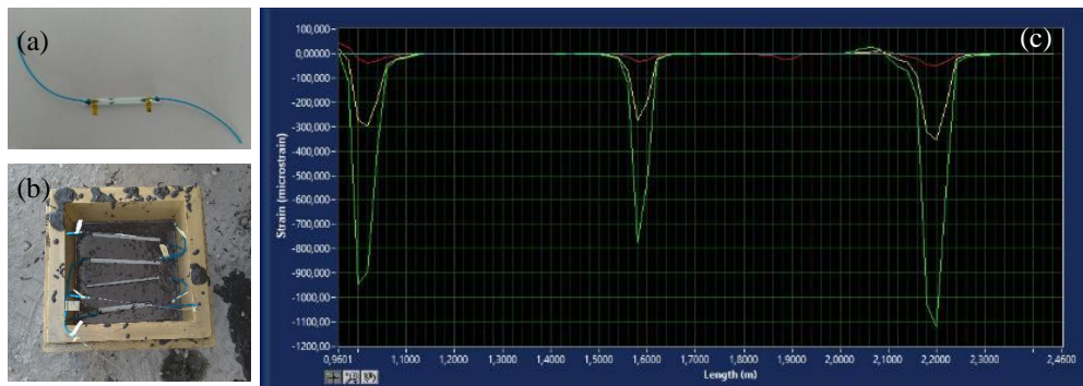
Figure 6: (a) SMART FRP rebar; (b) SMART concrete cube for compression tests; (c) Measured compression strain signals
